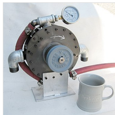
Quasiturbine QT-SC configured as a steam engine
